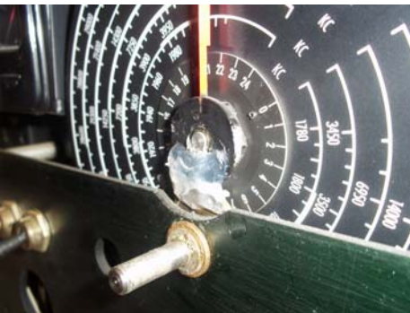
Right pointer wheel repaired and re-installed.
