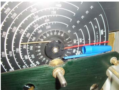
Right pointer wheel repaired and re-installed.
