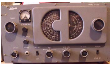
Lafayette KT-200, general coverage receiver, broadcast band through 30 MHz
