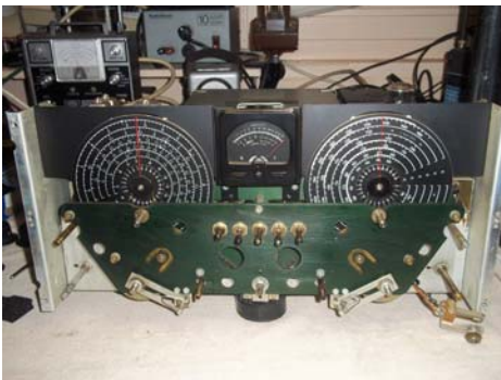
Right pointer wheel repaired and re-installed.
